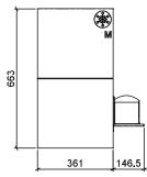
Cooling compartment size L Depth: 537 mm Inside dimension(W× H × D) 600 × 500 × 400 mm
